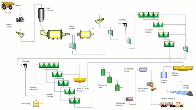
Figure 6 – Schematic of proposed flowsheet
