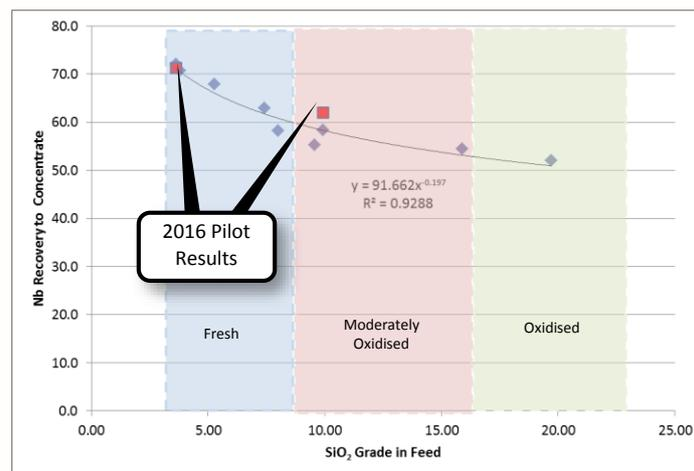
Niobium Recovery Trend by Geological Zone (SiO<sub>2</sub> Grade in Feed)
