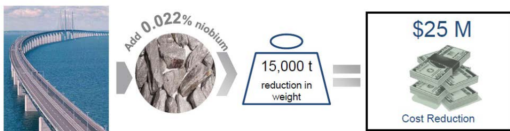
Figure 6: Construction industry cost benefits of niobium alloying in steel (Source: www.iamgold.com)
